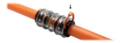
• If locking clips have been removed, please install the correct locking clip after connecting the microduct. By inserting the locking clip between the connector main body and the collet any possible microduct accidental disconnection can be avoided.
