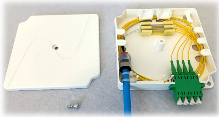
7/3,5 mm microduct and 4F micro cable installed to Nestor OptoBox 4 LC/APC 4xSMT pigtail kit
